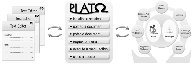
Figure 1: Architecture of the integration of the text-editor \text{TEX}_{\text{MACS}} and the \Omega\text{MEGA} system via the mediator \text{PLAT}\Omega
