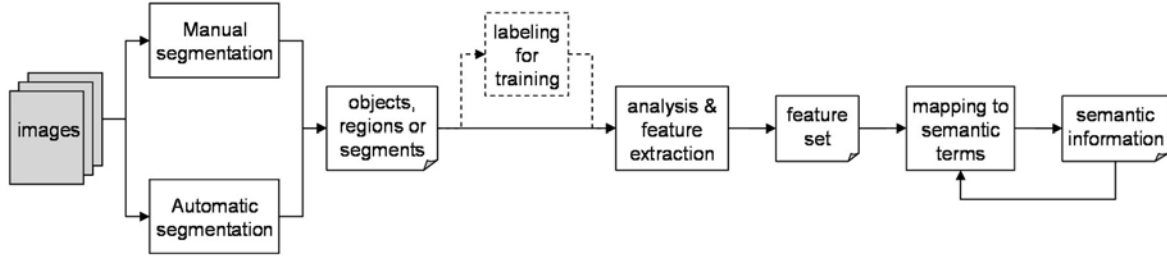
Figure 4: Generic process chain for image annotation or classification
